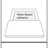
**5.** Broom or brush over the membrane to smooth it out and remove air bubbles.
